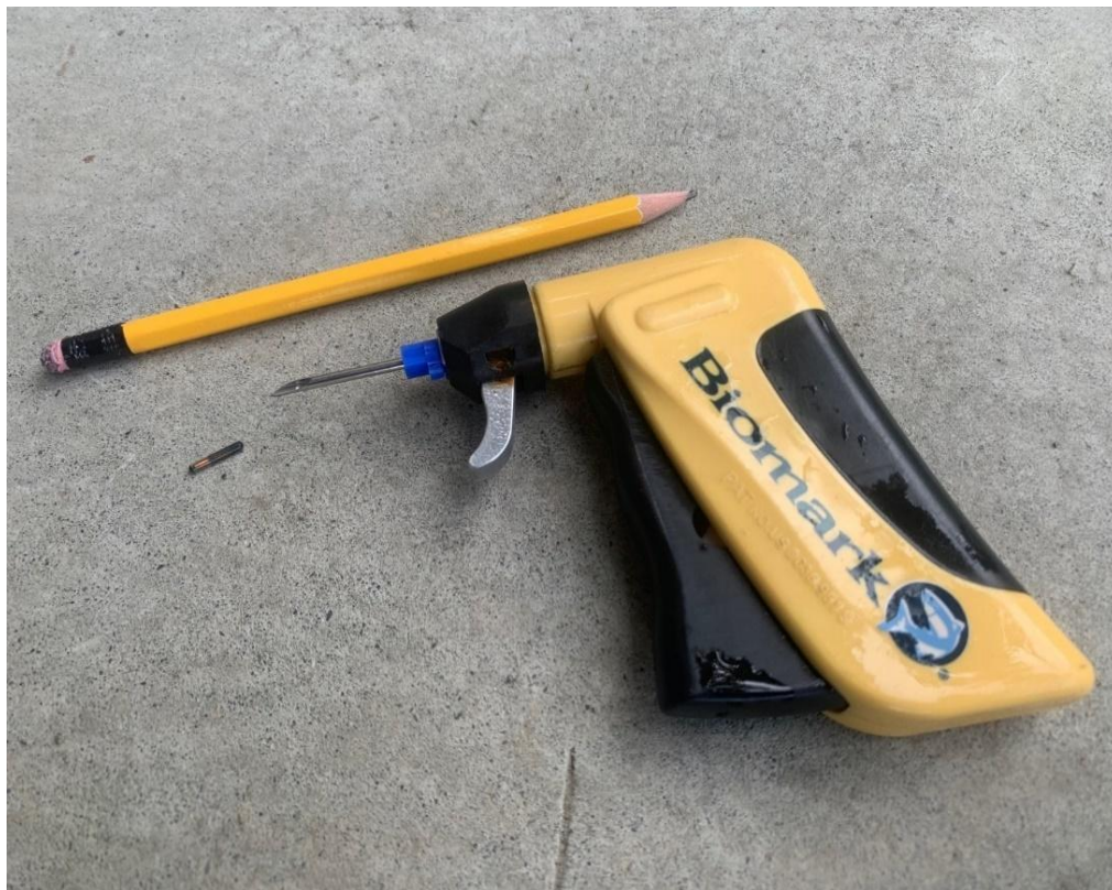
Figure 13: Biomark MK25 Passive Integrated Transponder tagging gun with an APT12 tag. Pencil is shown for scale.
