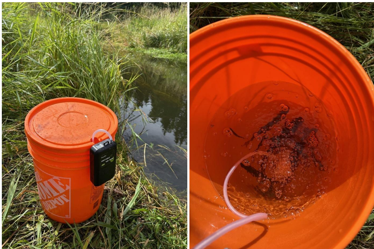
Figure 11: Holding bucket equipped with an air pump and air stones for oxygenation and a lid to prevent fish from leaping from the bucket.
