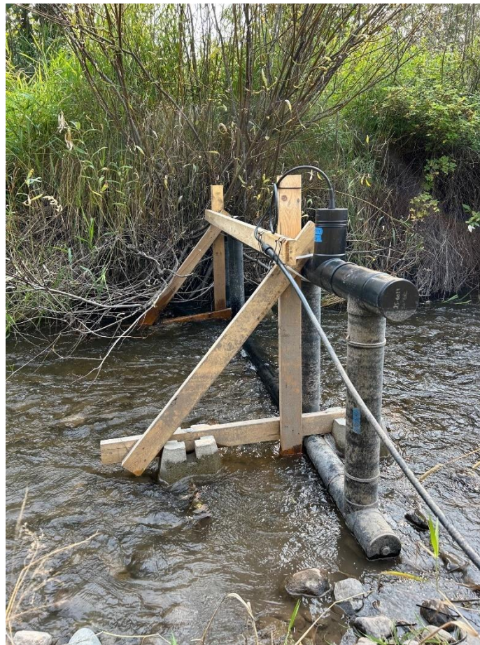
Figure 7: PIT detection antenna and bracket at the Clear Creek confluence site, September 2025. Note the algae on the antenna – the top of the algae was the water level during the Summer Temperature Management Program. Rope bridal not shown.
